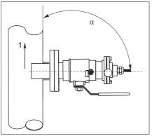
Installation with retractable assembly
