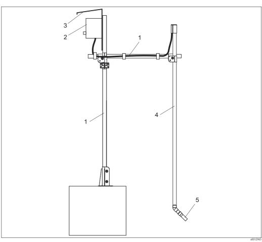
Measuring system with immersion assembly (example)
