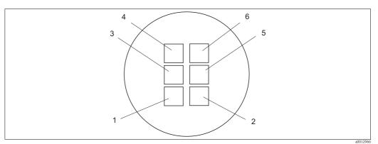
Arrangement of the light souces and the light receivers
