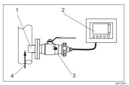
Measuring system with retractable assembly (example)
