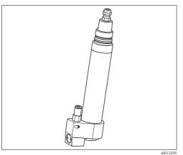
Cleaning system with pressurized air Consumption: 50 l/min (13.2 gal/min) Primary pressure: 1.5 to 2 bar (22 to 30 psi) Connection: 6/8 mm or  $6.35 \text{ mm} (\frac{1}{4})$
