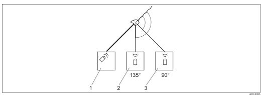
Principle operating mode of the turbidity sensor
